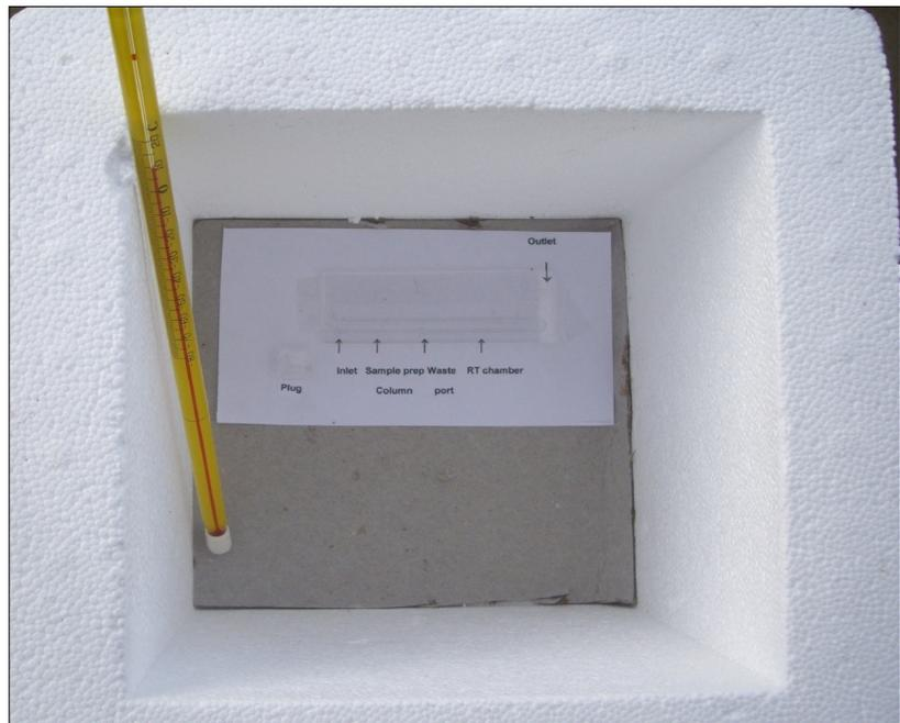
Figure 8. Styrofoam box containing the HT microfluidic device and a thermometer
