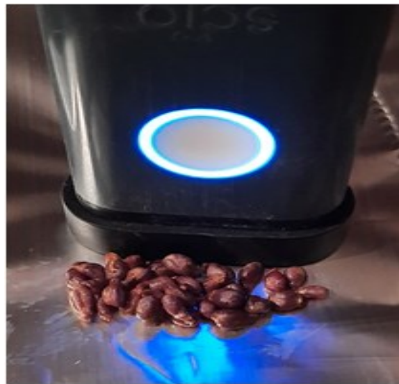
Figure 2. SCiO™ device being used to scan the 30 grape seeds.
